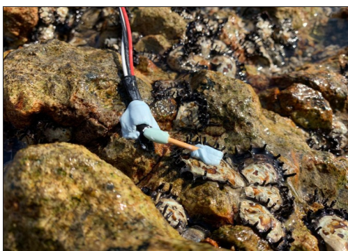
A hall-effect sensor on the shore to detect movement in rock oysters
