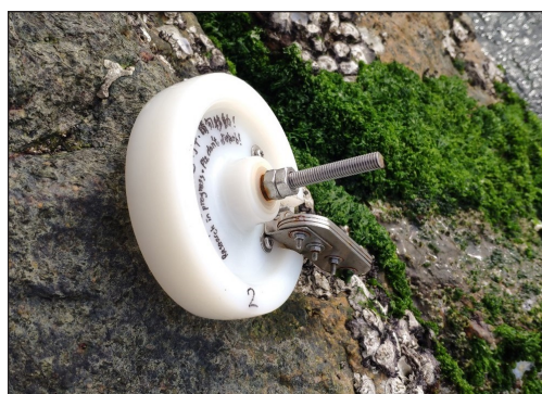
A deployed wave-logger on the rocky shore at Lung Kwu Tan
