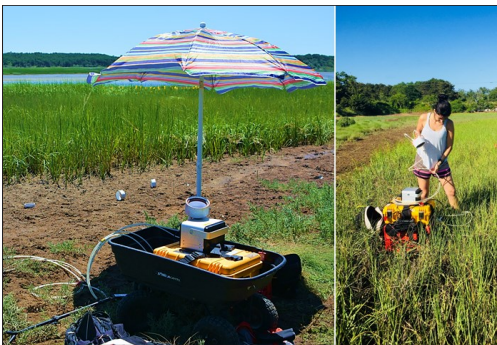
Laura performing greenhouse flux measurement within a NE-American salt marsh
