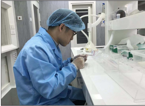
Oliver preparing chromatography columns to separate U and Th isotopes
